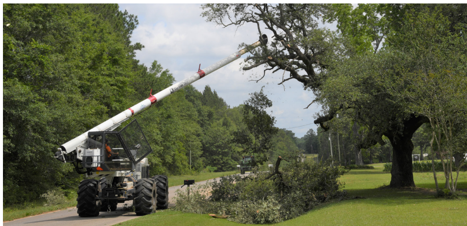
Southland's SkyTrim tree trimmer can extend to cut up to 75 feet high.
