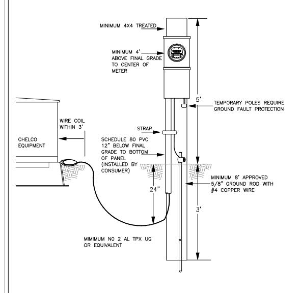
SPECIFICATIONS FOR SINGLE PHASE UNDERGROUND TEMPORARY METER POLE
