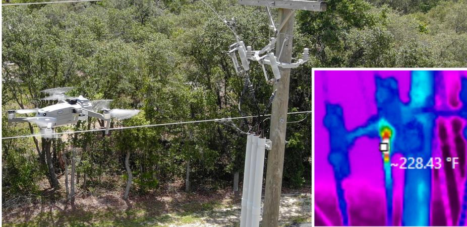
*Pictured above: A CHELCO Power Quality Technician captures a heat anomaly thanks to a drone equipped with infrared technology.*
